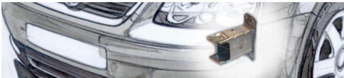
Figure 2. Crash box and its position in the car, behind the bumper on each side (illustration only)
