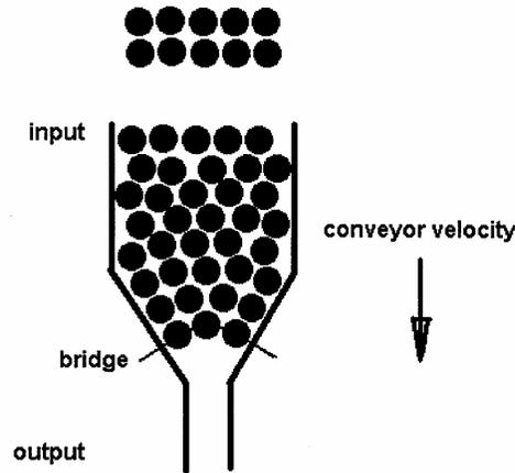
Figure 2. Arch formed from cylindrical components.
