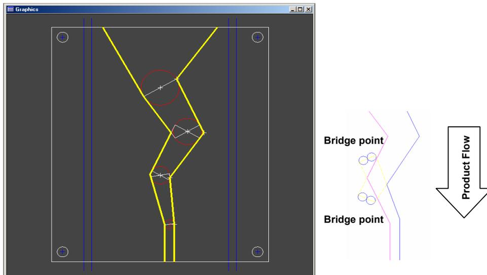
Figure 10. Zigzagging track to break up bridging.
