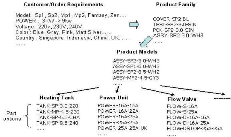
Figure 4. Product model and available configuration elements
