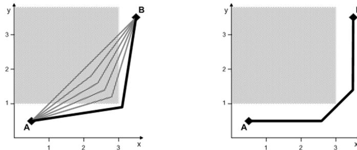
**Figure 7. Optimisation of structure-topology: two solutions**
