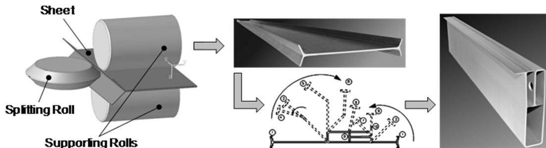
**Figure 1. Manufacturing multi-chambered profiles**
