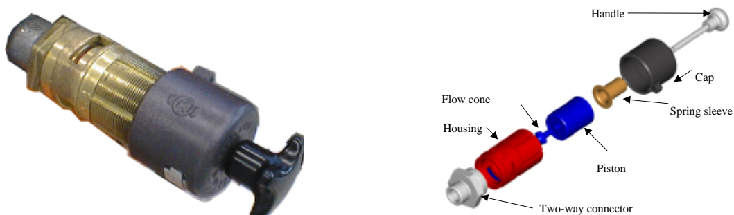
Figure 4. Picture and diagram of original design – main components marked [Lindemann 2001]
