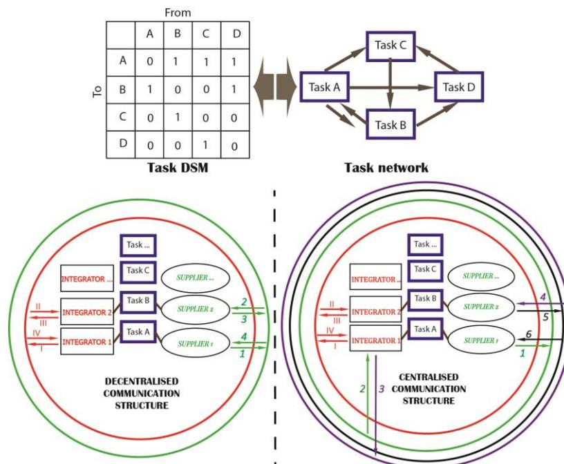
Figure 1. Decentralised (bottom left) and Centralised (bottom right) communication models with related task DSM (top left) and task network (top right)
