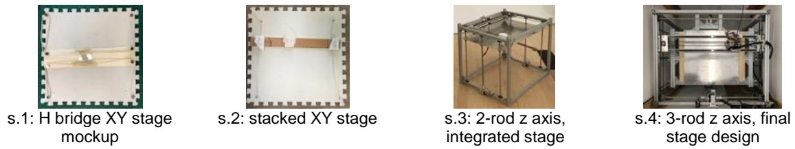
Figure 14: Search strategy for FDM x-y-z motion stage
