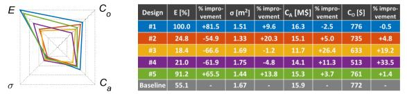
Figure 6. A spider plot (left) and the values (right) of the objectives for the five studied designs.
